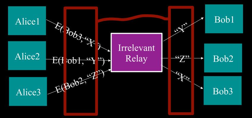
Timing analysis bridges all connections through relay  $\Rightarrow$  An attractive fat target
