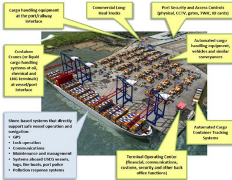
FIGURE 2—TYPICAL SHORE-BASED MARITIME ICS 23
