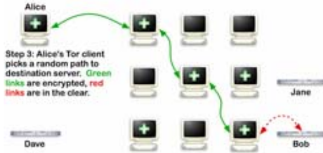
Figure 11. Message being bounced through several nodes on the Tor network. [Dingledine/Mathewson/Syverson 04]
