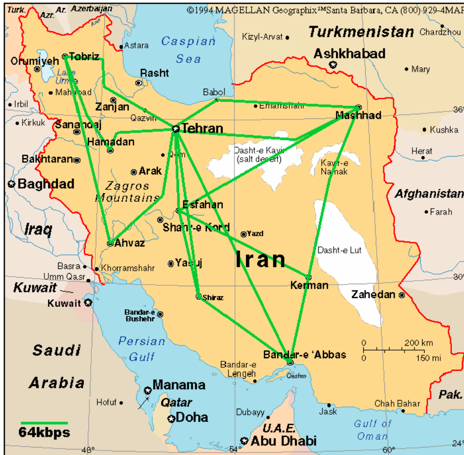
Figure 2. Iran’s inter-city ISDN lines as of 1997. This network has since been expanded to include other cities such as Yazd, Zahedan, Arak, and Rasht [ORN 99]
