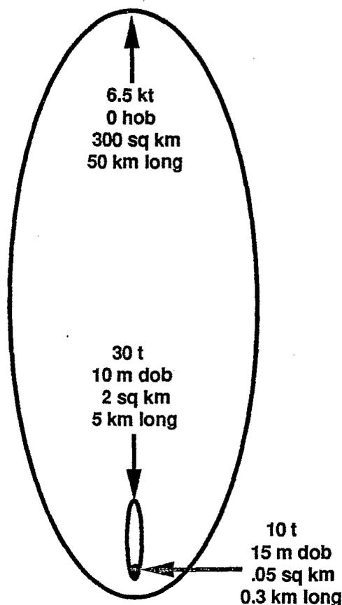
Figure 4 Relative fallout areas from three equally-effective nuclear weapons
