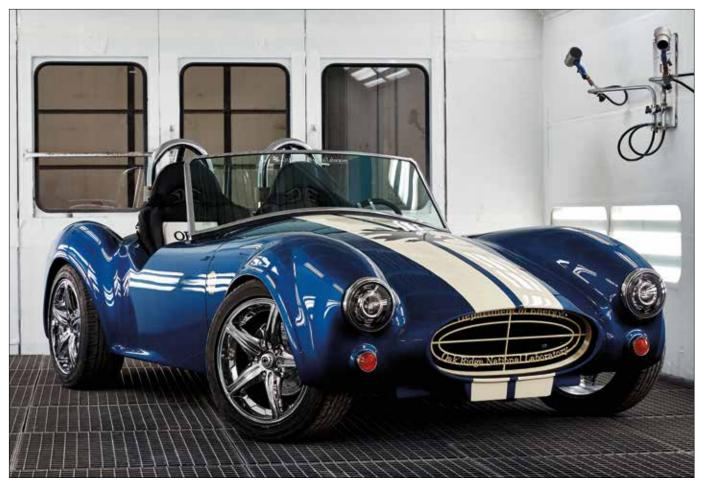
Shelby Cobra—approximately 1,400-pound vehicle containing 500 pounds of printed parts made of 20 percent carbon fiber—produced by Big Area Additive Manufacturing Machine, which manufactures strong, lightweight composite parts in sizes greater than 1 cubic meter (DOE)
