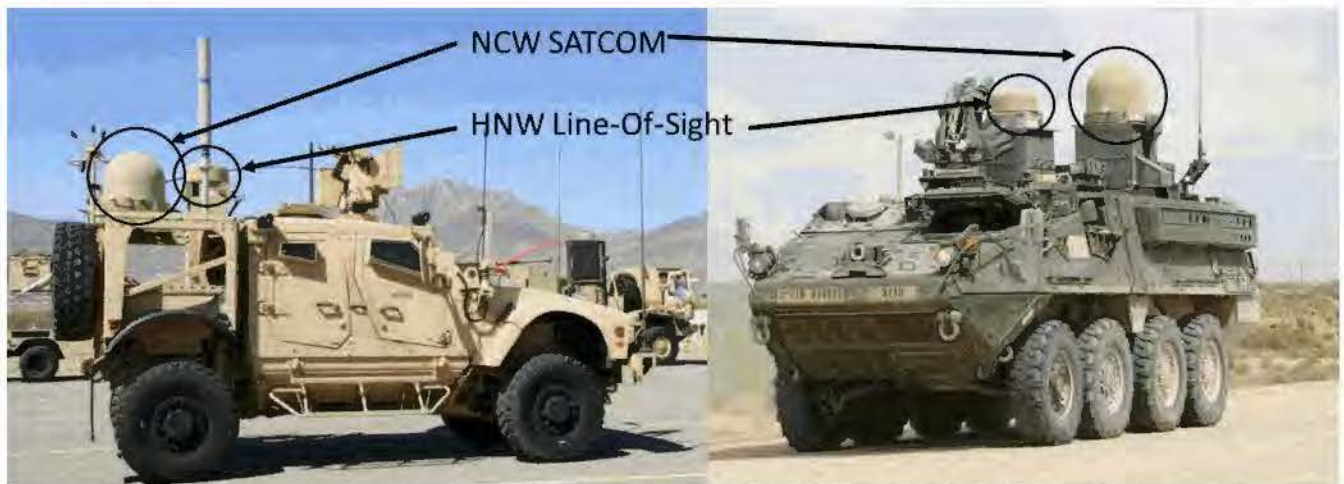
NCW SATCOM – Net-Centric Waveform Satellite Communications; HNW – Highband Networking Waveform Figure 1-2. WIN-T Increment 2 PoP, Installed in an MRAP All-Terrain Vehicle (M-ATV). Left: Integrated onto the MRAP. Right: Integrated onto the Stryker
