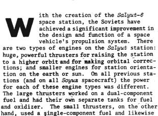
The Salyut-6 station, however, has a single dual-component fuel for both its large and small thrusters and fuel tanks for these engines.
