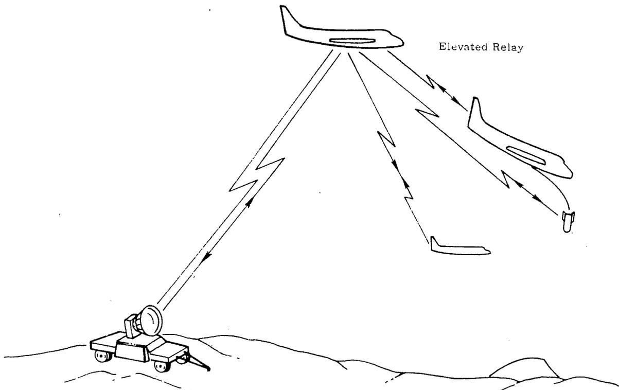
Figure 1. Elevated Relay Operation
