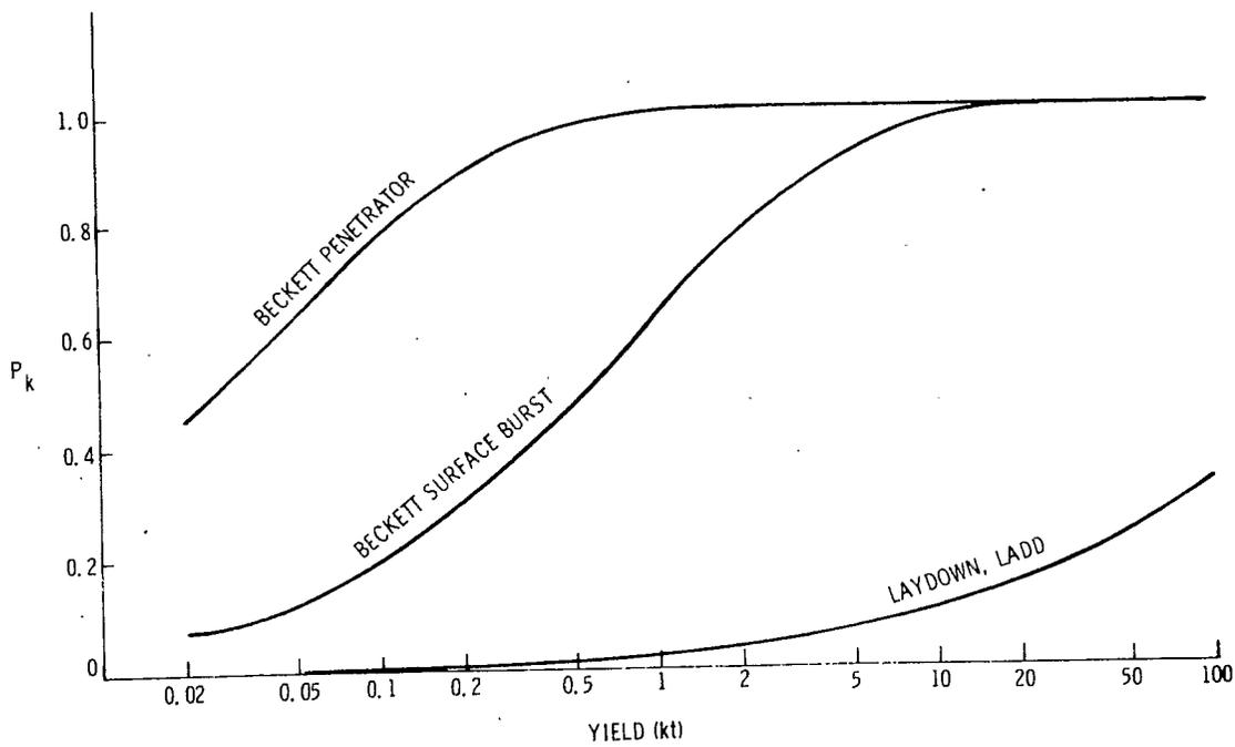
Figure 18. Hard-point target,  $p_k$  versus yield
