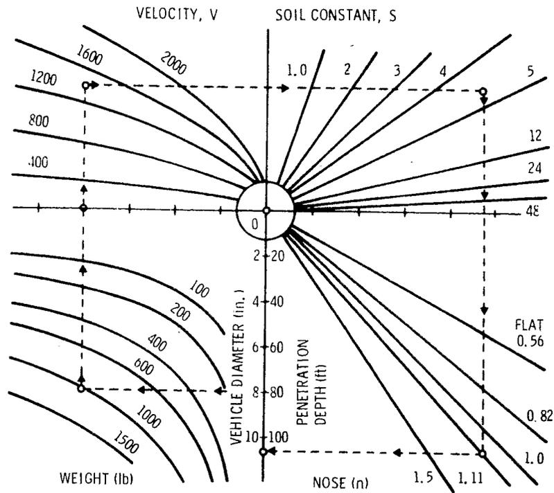
Figure 4. Earth penetration nomogram
