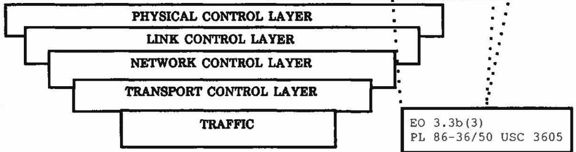
FIG. 2. TYPICAL LAYERS OF DIGITAL COMMUNICATIONS PROTOCOL
