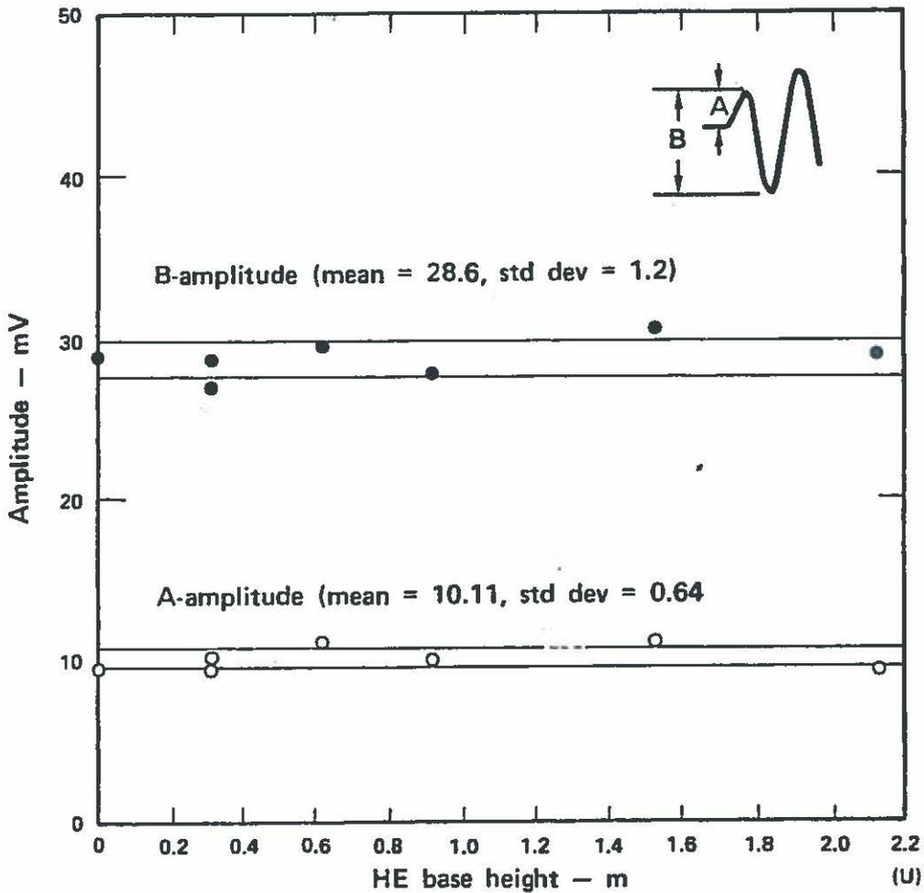
Figure 20. Amplitudes of the P-wave vertical velocity signals (see inset) recorded at the Linac Road seismic station vs the base heights of the 23-kg Comp. C-4 charges detonated in the KSO and KSC series of experiments. The horizontal lines are at  $\pm 1$  std dev from the mean amplitude.
