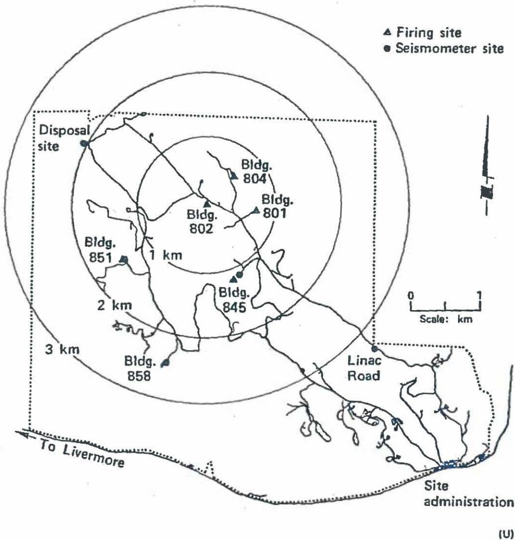
Figure 16. Seismometer emplacements at LLL's Site 300 HE test area.
