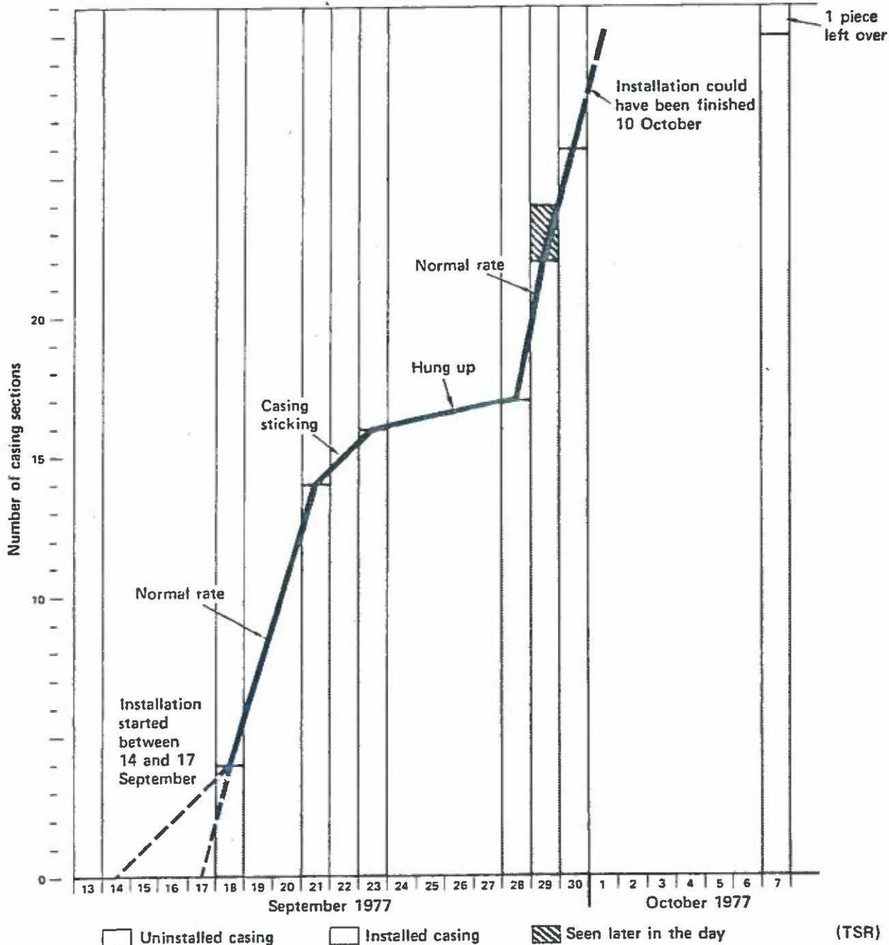
Figure 9. History of drill site casing installation.
