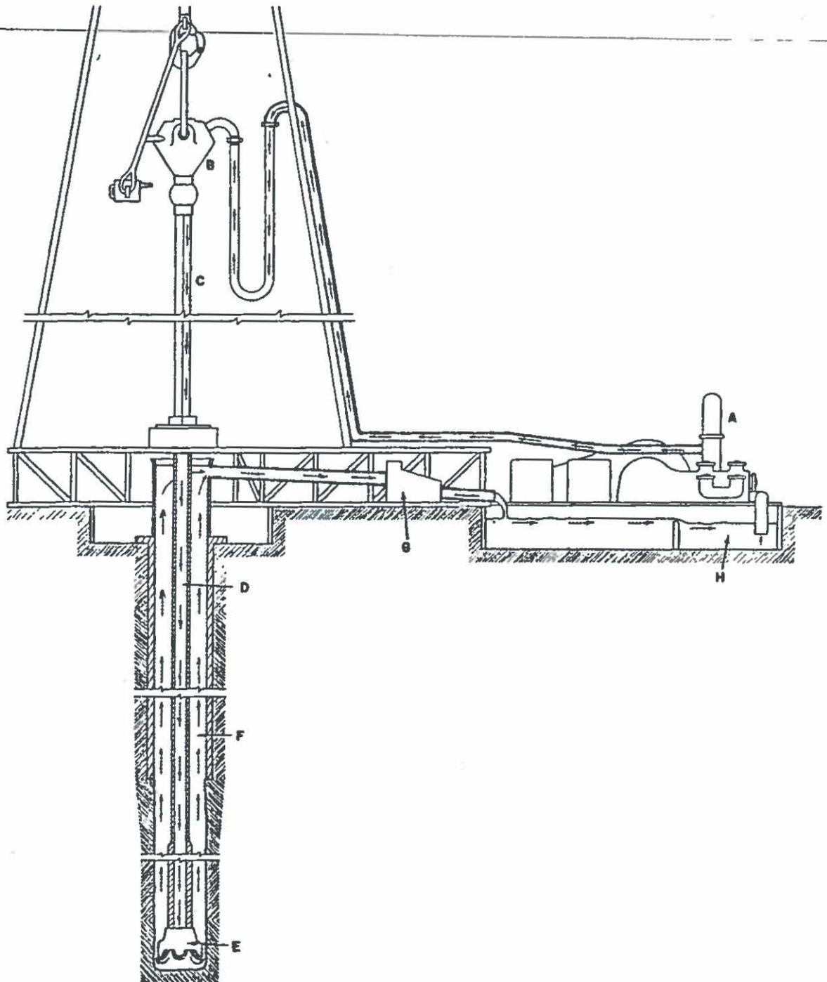
Figure 7. Circulation method believed to have been used at the Kalahari drill site. Arrows show path of drilling fluid: from slush pumps (A) to swivel (B) down through kelly (C) through the drill pipe (D) to bit (E). Fluid washes cuttings from hole bottom, carrying them to surface through annulus (F), through shale shaker (G), to mud pit No. 1 (H), on to pit No. 3 (not shown), from which entire cycle begins again.
